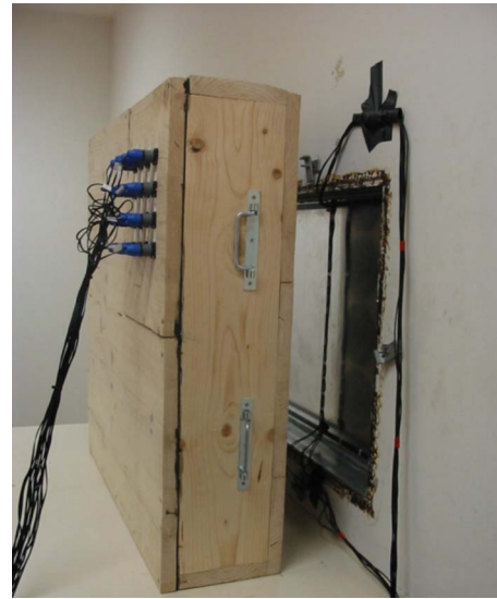
FIG. 5. (Color online) Photograph of the near-field array of loudspeakers for the synthesis of an acoustic diffuse field on the source room side of the test partition for the new methodology.
