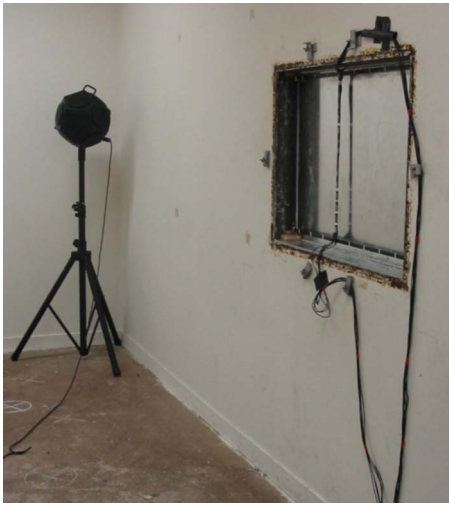
FIG. 4. (Color online) Photograph of the acoustic source and the test partition for the classical methodology.
