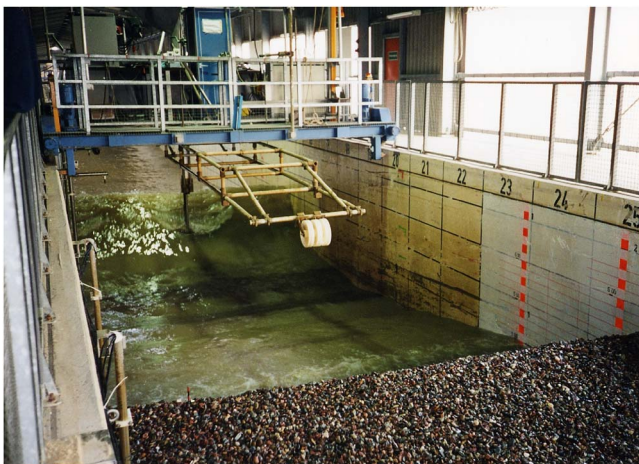
FIG. 2. (Color online) GWK viewed from beach end, showing mobile gantry with instruments submerged (the roller was used to profile the beach in between wave tests).
