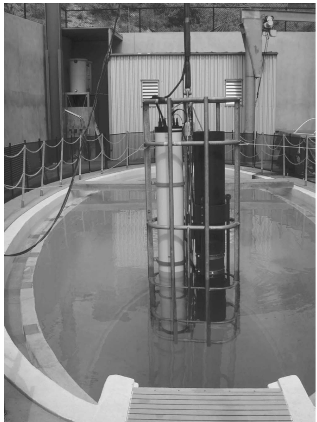
FIG. 8. Low frequency deepwater sound source in the SCRIPPS testing pool.
