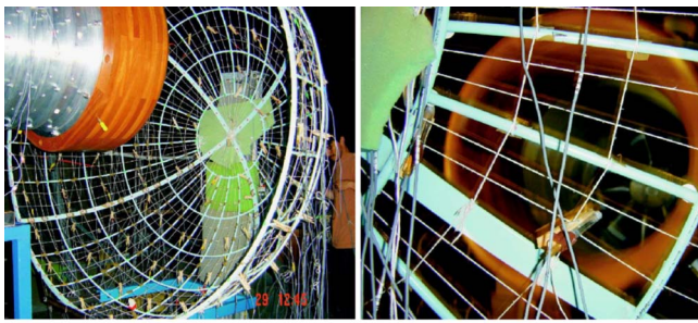
(a) Microphones mounted on the TCS (b) Close look of a microphone clipped on the TCS
